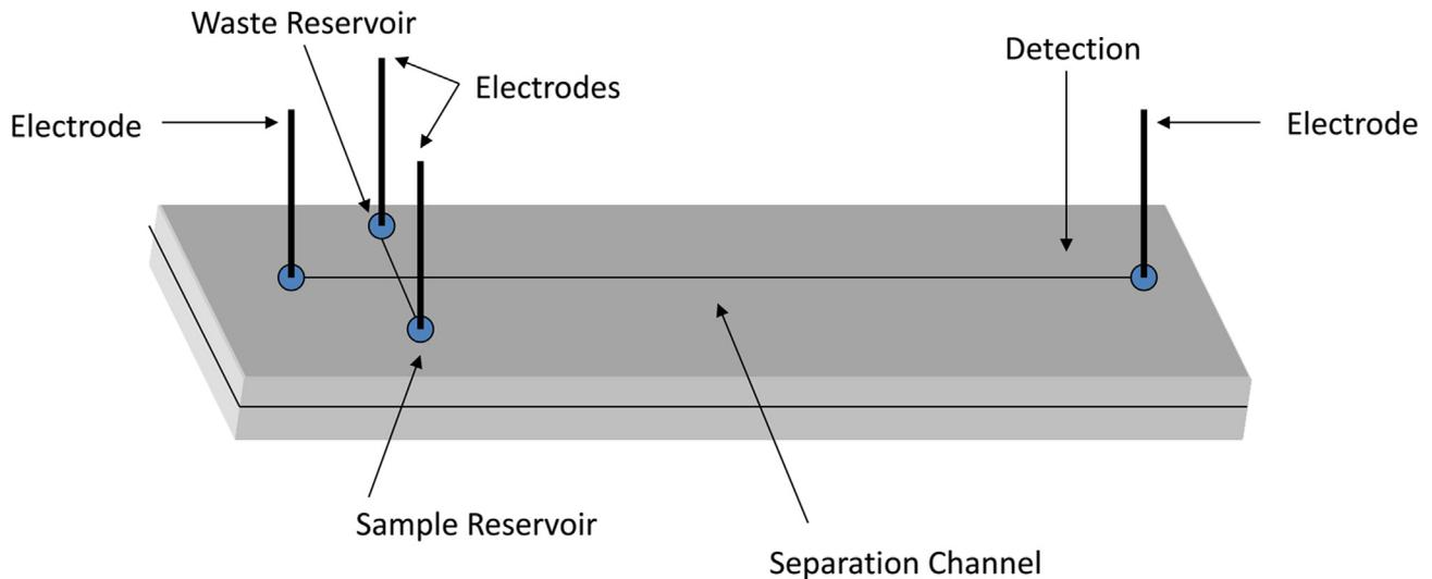
**Figure 1.** Microfluidic device for electrophoretic separations. Figure provided through the courtesy of Rose-Hulman Institute of Technology.
